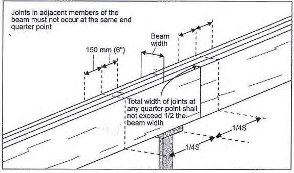
Figure 3.13 Nailing of Built-up Beams
