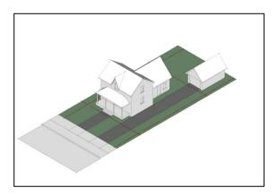
The above and left illustrations show recommended forms and setbacks for additions that are located to the rear of the building. Potential locations for new garages or ancillary structures are also depicted. A key consideration is that outbuildings are subordinate to the main structure (i.e. 3-car garages would not be an appropriate scale), and that open space is retained on the property.
